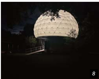
Figure 6: Test inflation of the finalised translucent envelope © Canobbio
